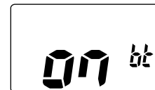
Battery voltage indication ON
